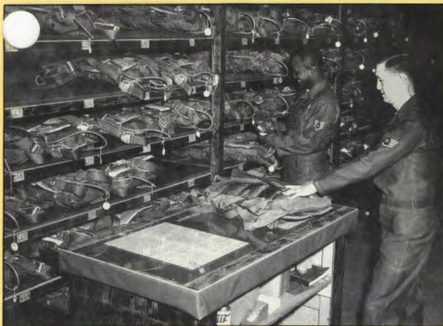
Staff Sergeants McGowan and Towers inspect back-pack parachutes using a locally-designed portable work stand. The stand contains the technical orders and equipment required for inspections and displays a check list on the top for easy reference while work is in progress.
